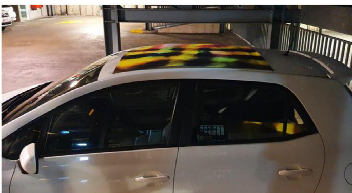
Adversarial patch on the roof of a car
