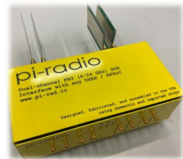
Pi-Radio FR3 board: 2x2 MIMO from 6.5 to 22.5 GHz
