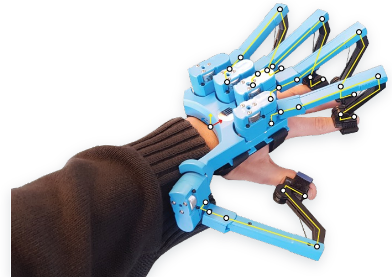
SenseGlove DK1.3 exoskeleton data glove.
