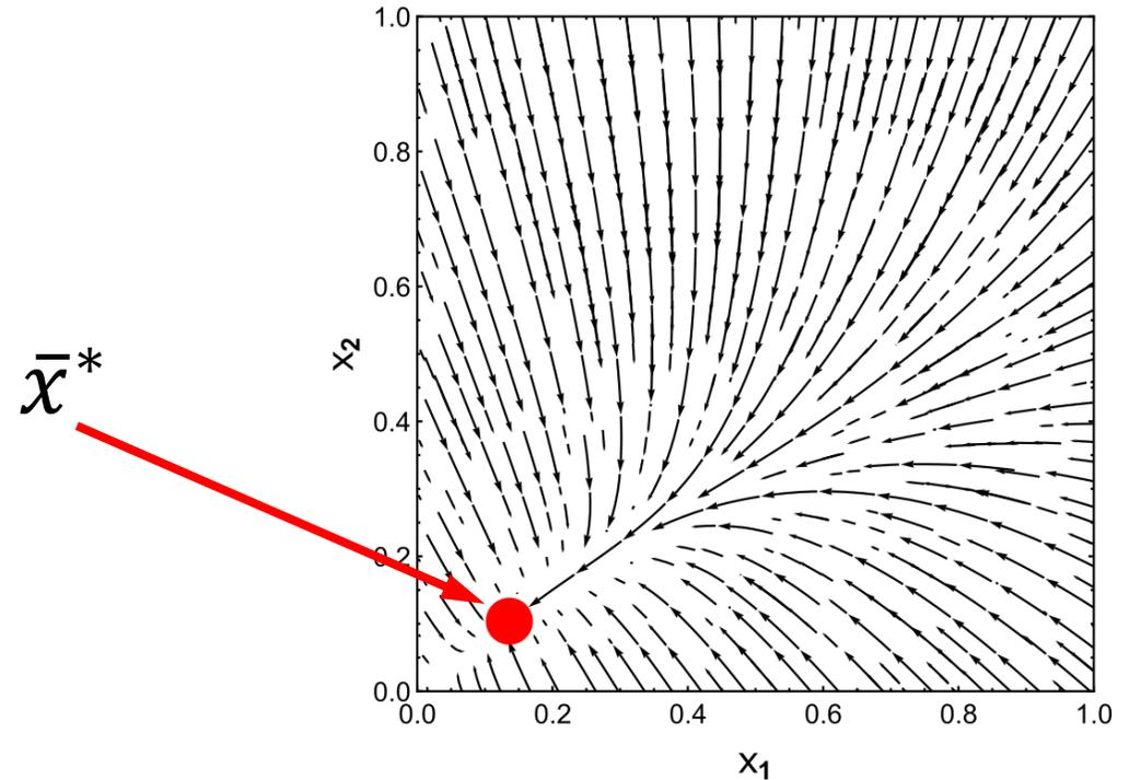
Controlled network,  $h_1 = 0.5x_1^{0.5}$ ,  $h_2 = 0.9x_2$
